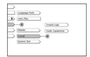
If you inserted an optical digital cable to the DIGITAL AUDIO OUT jack on the back of your player, you must set the *Audio Equipment* setting to *Dolby Digital* or *DTS* to match the brand of receiver you've connected to the DVD Player.
